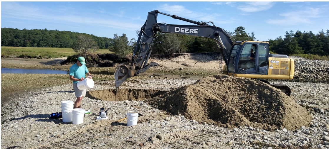
Consultant Trey Ruthven and Contractor Jason Richmond dig sediment samples at the Ellisville inlet.
