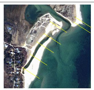
Aerial view of Ellisville Beach and Ellisville Marsh tidal inlet channel showing locations of transects that have been set up to enable low cost monitoring of barrier beach elevations on an ongoing basis.
